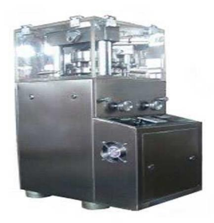
This machine is single pressing and capable of automatic revolution and continuous pressing to press raw material in particle from into tablets. It mainly applies to the tablet production in pharmaceutical industry and also is applicable to chemical, food, electronic and etc.
