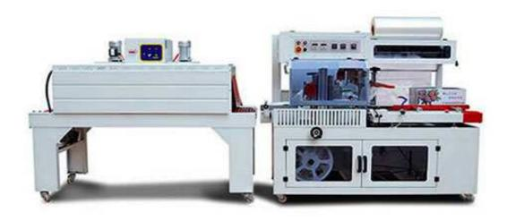
PZS-1050L automatic heat shrink packaging machine is a fully automatic unmanned operation "L" automatic shrink packaging machine, widely used in food, pharmaceutical, daily chemical, hardware, electrical and other industries, especially mass production. Packing flow operation, high work efficiency, automatic film feeding and punching device and manual adjustment of the film guiding system and manual adjustment of the feeding platform for different widths and heights.
