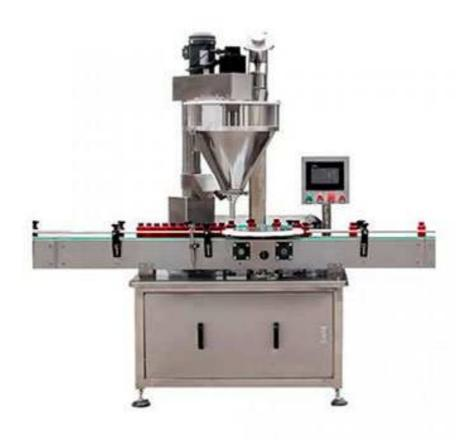
Applies the latest technology, meet with the latest national GMP standards. Reasonable design, simpler and stronger. It can automatically complete the measuring and filling, suitable for packaging powdery products such as medicine powder, milk powder, protein powder, chicken powder etc.
