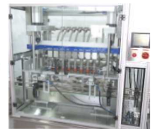
機台安全外罩 Machine safety cover
