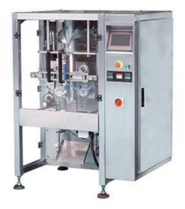
The machine can be used for powdery and granulated material such as milk powder, solid drink, white sugar, dextrose, fodder, pharmaceuticals, agriculture pesticide, granular additive, dyestuff, etc. material automatic packing into bags with high speed and accuracy.
