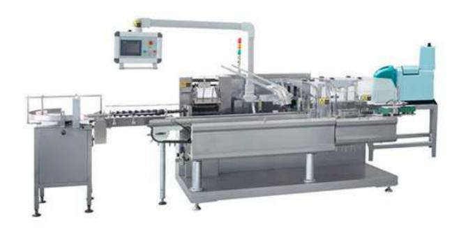
This machine is suitable for automatic feeding and packing round bottles or items into folding carton. This machine can automatic convey bottles, fold leaflet (1 to 4 folds), convey and detect leaflet, absorb folding carton, form and convey them, put items into carton, press batch number, close and seal carton, or use glue sprayer or hot melt glue machine to seal carton according to requirement, reject unqualified product, convey finished products out.
