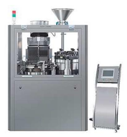
With an output of 3800 capsules per minute, the processing range of the NJP-3800C includes (micro) tablets, powders, pellets, and granules. The NJP-3800C is a flexible capsule filling machine that provides a high versatility of filling options with varying product types. Even complex products with varying filling parameters can easily be processed.
