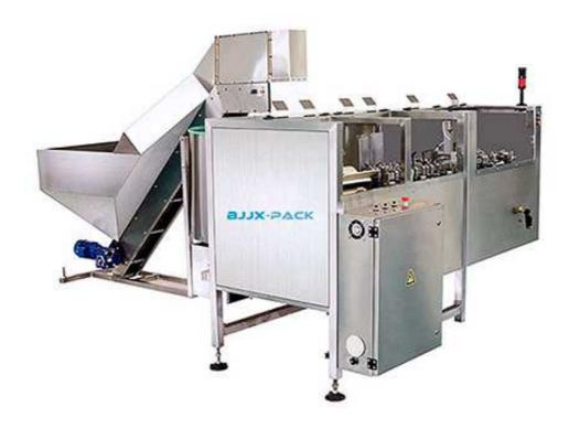
This machine is used for arranging disordered polyester bottles. Randomly oriented bottles are received in bulk into the hopper and supplied to the centrifugal disc by means of a conveyor. In the disc, the bottles are guided into a qualified position suitable for the stand.
