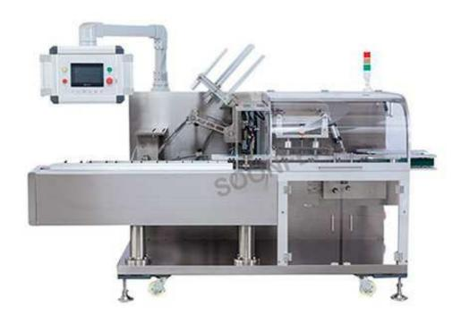
Carton box packing machine is designed with box forming, feeding, folding, glue spraying and sealing systems.
