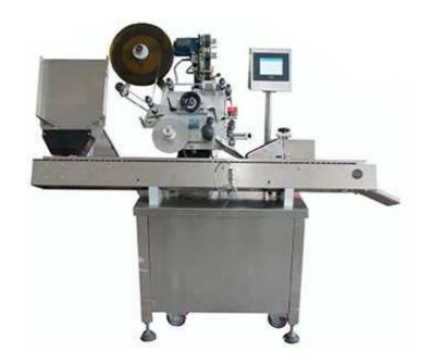
DWTB-C is economical, self contained, easy to operate, equipped with auto teach programming touch screen. Built in microchip storing different job setting makes fast and easy changeover. This automatic labeling system is ideal for slim cylindrical container with diameter from 10mm-25mm such as ampoule.
