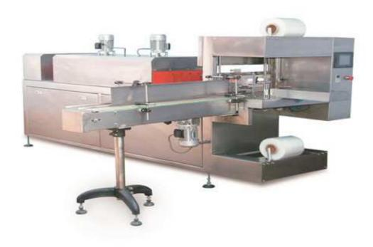
The machine is widely used in mineral water, beverage bottles, beer bottles, cans and other multirow tray packaging. Can be used with automatic filling machine.
