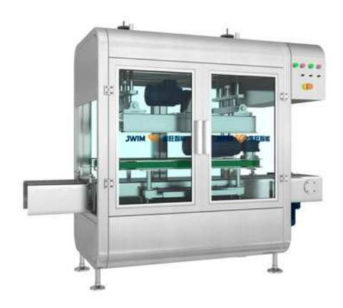
YG-260 roller type capping machine mainly adopts the mode of manual cap placement and automatic cap pressing. Automatic capping can be effectively carried out through roller conveying (Two belts clamp the pail, top roller press the cap).
