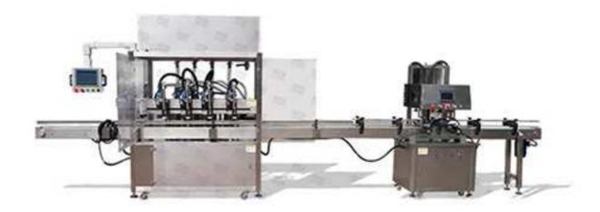
Our double head liquid filling machine is made of all 304 stainless steel, and 316 stainless steel can also be customized. This machine has simple structure, high filling precision and convenient operation. This filling machine is widely used in liquid filling in food, daily chemical, pharmaceutical and other chemical industries.
