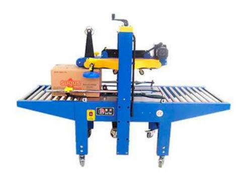
FJ6050 carton sealing machine is mainly used in sealing and packing cartons, which can be used either independently or as a necessary part of a production line. The machine is widely used in the fields of electrical, domestic, textiles, foodstuffs, general merchandise, medicine and chemical industries.
