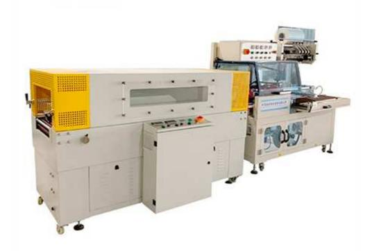
Shrink Tunnel Machine L Bar Sealing Machine are available in both automatic and semi-automatic formats. L-Sealers are perfect low volume shrink packaging solution able to seal up to 30 packages a minute.
