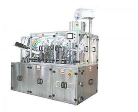
Automatic Linear tube filling Machine is precision built on sturdy welded MS frame completely enclosed in stainless steel sheet and doors are providing to facilitate the servicing of machine.
