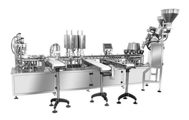
The CapperPacks Automatic Bottle Filling Capping Machine is suitable for candy and other granule filling and packaging. It features the dual-station index vibrating filling system and user friendly control system with PLC and touch screen interface.
