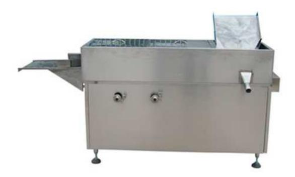
This machine is the cleaning equipment in the oral liquid production line, which Is mainly applied in the cleaning of straight tube bottle with 5 to 20 ml EPOL, Aluminum plastic combined lid (or safety lid). This machine transports the bottle by screw, and the bottles are double cleaned Inside and outside with pressed recycled water, ionized water (or other washing Solution). Then blew off the left water with purified compressed air.
