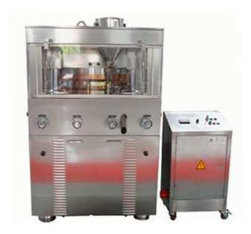
This machine is a double-press type; it continually and automatically tablet press granular raw materials into round tablet, irregular tablet, carved tablet and two layer (color) tablets etc. It is mainly used in pharmaceutical industry and also the chemical, food, electronic industry and so on.
