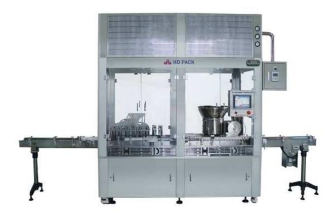
HD-VFW Series are monoblock vials filling and sealing machine with continuous motion of positive monoblock transport system and suitable for filling liquid solution into cylindrical vials, rubber stopper insertion and aluminum sealing. HD-VFW Series are very compact and carry out multifunctional performance from filling to sealing in a single rotation, ensuring maximum production efficiency and safety.
