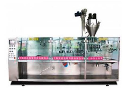
As regard to the 3 and 4 side sealed small sachets, the duplex design increases the packaging speed by 100% without adding additional costs. The machine can be used to package milk powders, coffee powders, condiments, granular materials, ketchup, shampoo etc.
