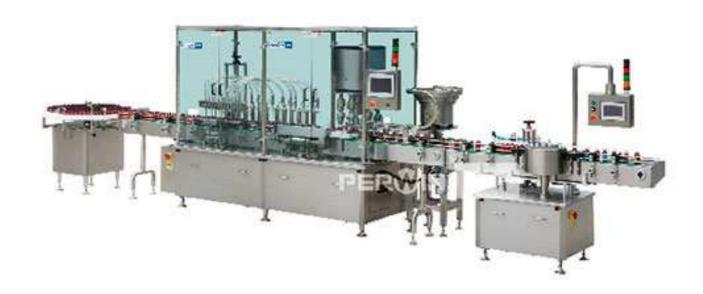
It can be applied to 10~100ml, 150~1000ml round bottle or cubitainer (rectangular cubitainer), 2L~6L cubitainer (rectangular cubitainer), and big volume buffer solution, cleaning solution, diluent and so on.
