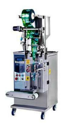
Sauce Sachet Filling Machine is suit for automatic filling and packing liquid/paste/sauce/cream item, such as milk, honey, hair shampoo, tomato paste, salad dressing, jam ect. Sauce Sachet Filling Machine adopt the pneumatic pump dosing unit which have the machine advantage of suit for viscous liquid item with high efficient and reliable performances
