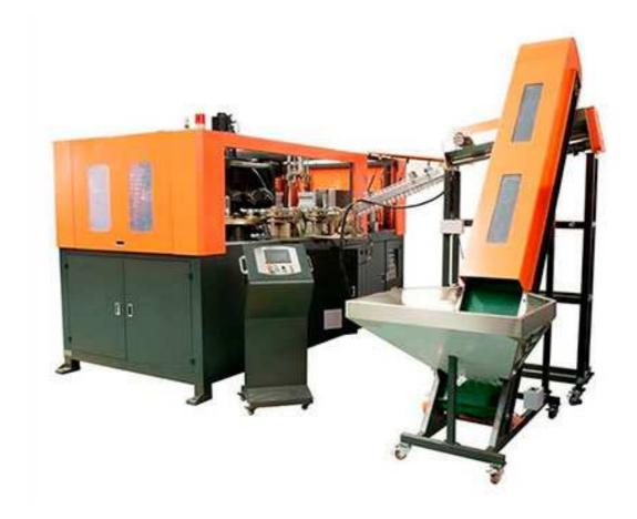
The Q3000 bottle blowing equipment is importing the preform, and through the high-precision handle pick-and-place device, it can be servo-positioned, quickly and accurately put the handle in the mold, and then blow the bottle, so that the bottle body and the handle are fully integrated, and the bottle is fully handled.
