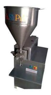
We specialize in deliver custom viscous filling machine that can be used to fill various products like bam, hot balm, wax, lip balm, cream etc in melting condition. We provide machines to fill viscous and semi viscous fluids in various types of containers. The machines are auto piston type that is rational in design. Our machines are popular providing disturbance free heavy duty performance and available at the most affordable rates.
