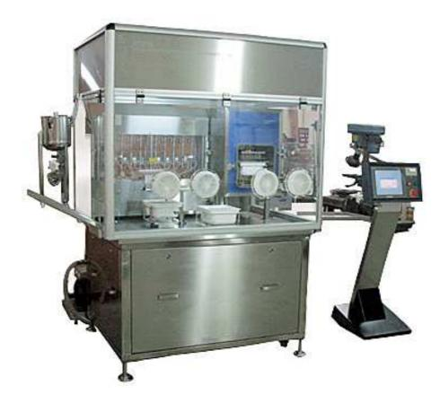
Model –PFS-SA-10 is very compact and elegant PLC. Based cGMP model for automatic filling and Stoppering operation of pre filled syringe.
