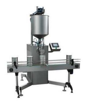
This single head sauce filling machine is suitable for sauce filling which can dia is 153mm. It adopts Fuji servo motor and servo motor controller to control filling valve route. User could change the filling volume between 400g and 4500g via touch screen continuously. High filling precision, error control within  $\pm 4\%$ .
