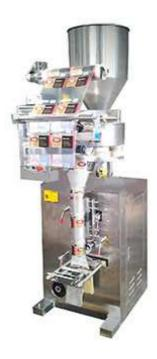
This machine is suitable for packing many kinds of powder, granule and so on. Mostly used in the daily life. For example, electuary, oatmeal, white granulated sugar, coffee, gourmet powder, condiment, milk powder, soybean milk powder, medicine powder, nettle, pepper and so on. This machine is fully automatic.
