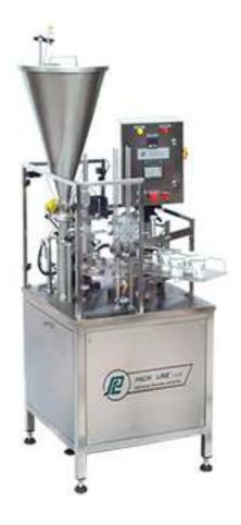
A fully automatic filling and sealing machine with pre-formed lids or membrane cut directly from roll. Rotary platform is driven by analogue engine. This filling and sealing machine easily handles up to 20 oz. of volume and utilizes 7 to 9 station rotation platforms depending on cup configuration and capacity. Two filling operations may be preformed in the same cup before sealing.
