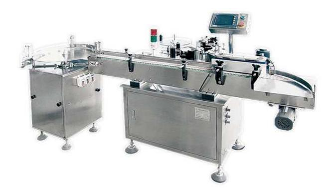
KTN-A non-dryer sticker labeling machine is improved from the same type at home and abroad. It can auto change label, auto check label, inspect bottle in-position, applies to label on cylinder straight tube bottle and plastic bottle. It's ideal equipment for pharmacy, food, chemical industry to label non-drying sticker.
