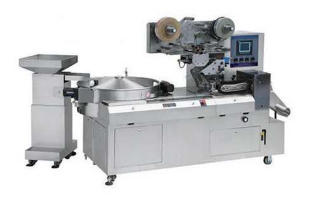
SGMZ800 Candy Flow Packing Machine suitable for wrapping all kinds of hard candies as well as other regular shape such as chewing gum, bubble gum and chocolate ball. The machine is fully automatic and is complete with a vibratory feeding disc & multi brush plate feed system. Print registration unit, wrapping counter & pack length change by keypad are all standard items. The maximum speed is up to 800 pcs per minute.
