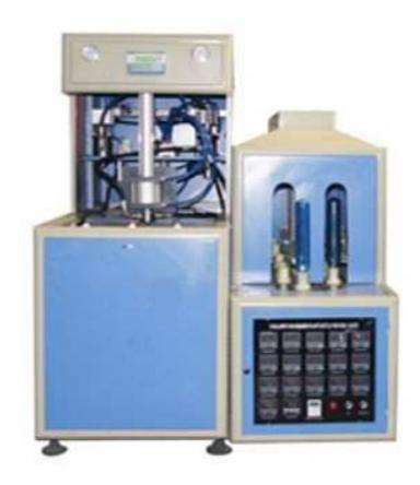
ES-5G two step manually preform inserted full auto bottle blower is applicable for blowing the carbonic acid beverage bottle mineral spring water bottle, farm chemical bottle, oil bottle, medical, hot-filled bottle in any shapes and made of PET raw material.
