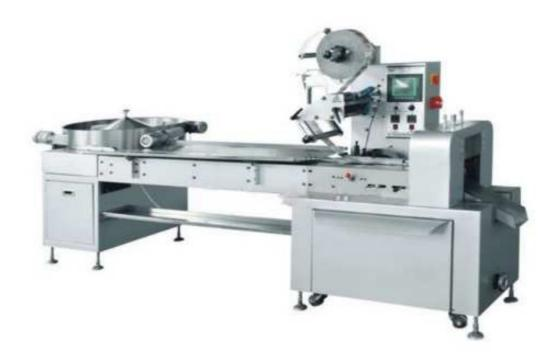
The material with uniform specifications can be sent to the bag-making machine through the automatic sorting tray for sealing and cutting, and the finished product output is completed automatically.
