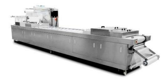
The Utien DZL thermoforming packaging line is designed for maximum output and used in food industry frequently. The new model of thermoformer redefined high durability and high work efficiency.
