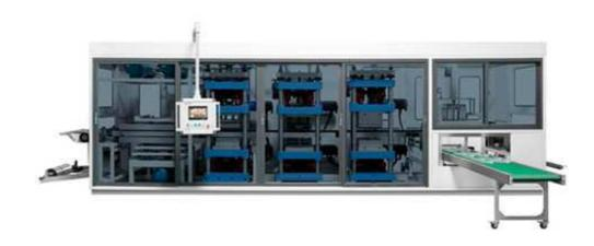
Automatic PS seeding tray thermoforming machine is used to producing different sizes of seeding trays, egg trays, fruit box, soap tray, flower pot and etc. The machine is completely driven by servo motor.
