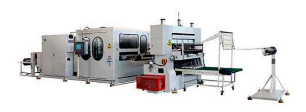
HSC-750850+HLQ-1000 FORMING & PUNCHING LINE adopts the most advanced plastic thermoforming technology and was developed to be a forming machine of high production efficiency. It is a combination of mechanical, electrical and pneumatic components, and the whole system was controlled by micro PLC, The machine has man-interface operation, radiant heat, male and female die forming and high speed punching. It combines feeding, heating, forming cutting, stacking and counting into one line station.
