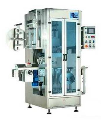
The shrinking machine gets the water supply from the bottled water. The float electric water level controller presets a figure, then water in the tank will be heated, when temperature up to the preset figure (4-7 degree adjustable), When the temperature of steam reaches to 140-170°C the machine starts to work.
