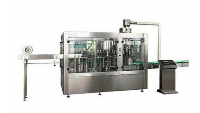
Mineral Water Filling Machine Factory in China combined water bottle washing, filling and capping into 3 in 1 monoblock. It is suitable for both plastic polyester bottle (PET bottle) and glass bottle with screw caps for non-aerated carbon dioxide drinks such as mineral water, pure water, non-gas water, spring water and so on. The water filling machine design could shorten the time for the drink material contact with outside, increase the sanitation condition through economy benefit.
