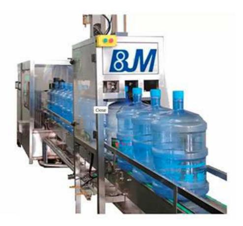
This automatic barrel washing machine can effectively wipe off the mineralization precipitate, and all-round washing the outside of the barrel, which increase the washing result and reduce secondary pollution of manual work as well as the labor intensity of operating worker. The main material is stainless steel which is corrosion resisting and easy to clean.
