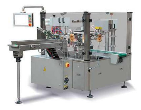
Rotary bag-given packaging machine with different dosing (such as multi-head weigher, liquid filler, auger filler etc.), can be suitable for the automatic packing for granular, powder, liquid, paste etc. Different kinds of products with the premade stand-up pouch with zipper.
