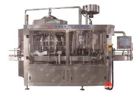
The rotary filling and capping machine is automated from filling, capping and bottle retreating, with simple operation and fast packaging speed. It can also change the template and capping head according to different bottles and lids at any time, and it is convenient to load and unload.
