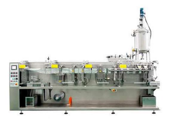
Liquid soap doypack filling machine can complete pouch forming, feeding, measuring, filling, sealing, date printing, nitrogen filling, counting, finished product delivery. It is suitable for filling different products such as powder, granule, tablets, liquid, cream and other non free-flowing liquid when equipped with feeding and measuring devices.
