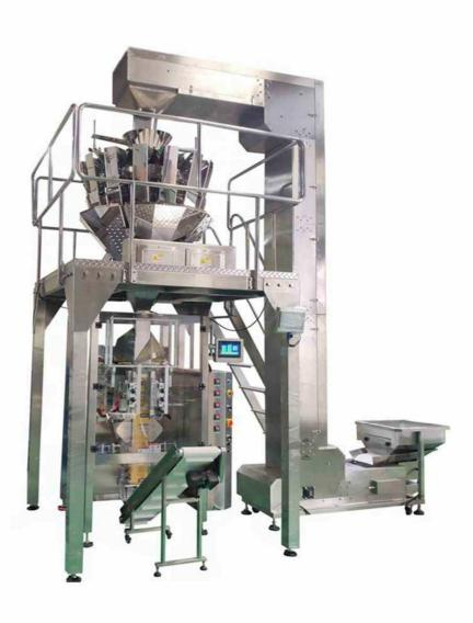
The gusseted bag packing machine is a high level bag design which looks much better than standard pillow bag, especially for supermarket selling; suitable for biscuit package, coffee with valve package, tea packaging etc. Also, additional punching, such as hole punching, euro punching, handle punching etc.
