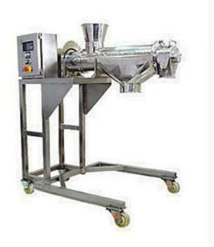
**PMS CENTI SIFTER®** is an innovative mechanical screening which offers high efficiency and throughput in various bulk solid processing for non-abrasive and non-friable materials. Its functions can be categorized into Scalping, Policing, Separation, Classification, Deagglomerating and Conditioning. The sifters are widely used in pharmaceutical, chemical, food, agricultural, plastic, chemical and agricultural industries.
