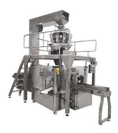
Full automatic premade pouch bagger, featured with rapid reaction, reliability and quick changeover, is ideal for a large variety of bag types and range. Equipped with Z-shape bucket elevator and combination scale, it is widely applied to candies, microwave popcorn, cookies, nuts, rice, coffee beans, crops, peanuts, etc.
