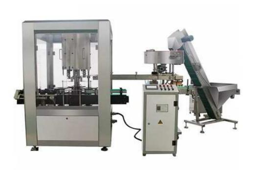
With 4 mechanical hands, the model is used for multi-geometry containers. It dispatches caps at high speed without any cap reversed. Cap supply system and mechanical hands work together in phase. When the cap is tightened, bottle and cap stand still relatively, and the clutch separates immediately so that cap and bottle are not apt to be damaged.
