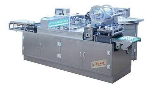
1. The length of the tray can be input in touch screen. Molds are located in positioning slot, and it's convenient to change the molds.
