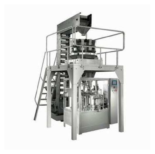
Granule packing line mainly installs preformed pouch packing machine, computer combination weighed, Z type material conveyor with feeder, working platform and product conveyor, which is suitable for packing solid, granule and so on. Our rotary pouch-packing machine utilize the latest technologies to achieve the steady speeds and most accurately packaging effect.
