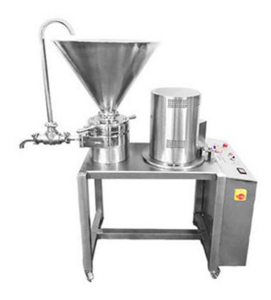
Colloid Mill is an ideal and perfect homogenizer-cum-emulsifier. It finds its application in various processes like grinding, homogenizing, emulsifying, dispersing, mixing, extracting etc., catering to the needs of several industries, such as
