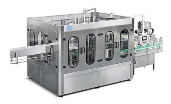
The large bottle water filling machine is especially used for large bottle size from 3L-10L. Large bottle water filling machine is welding by steel structure, supported by stainless steel adjustable feet, surface coating with 304 stainless steel layer for anti-corrosion function.
